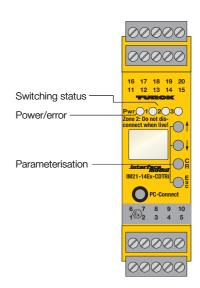
The rotation speed monitor IM21-14EX-CDTRI monitors pulse sequences, rotation speed and pulse trains of rotating motor, gear or turbine parts for over and underrange of programmed limit values. A display integrated in the front cover indicates the current value.
