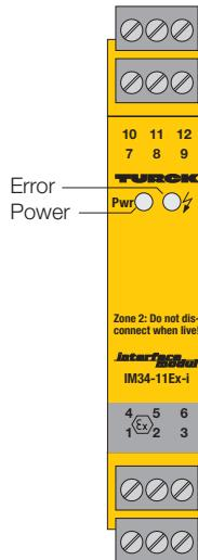
The temperature measuring amplifier IM34-11EX-I is designed to evaluate the temperature-dependent variations of Ni100/Pt100 resistance temperature detectors, thermoelement types B, E, J, K, L, N, R, S and T or low voltages in a range of -100...+160 mV and to output them as linear temperature current signals.
