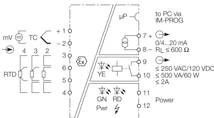
The 1-channel temperature measuring amplifier IM34-12EX-CRI is designed to evaluate the temperature-dependent variations of resistance thermo detectors (RTD) Ni100/Pt100, thermoelement types B, E, J, K, L, N, R, S and T or low voltages in a range of -160...+160 mV and to output them as linear temperature current signals.
