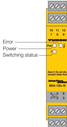
The 1-channel temperature measuring amplifier IM34-12EX-RI is designed to evaluate the temperature-dependent variations of resistance thermo detectors (RTD) Ni100/Pt100, thermoelement types B, E, J, K, L, N, R, S and T or low voltages in a range of 100...+160 mV and to output them as linear temperature current signals.
