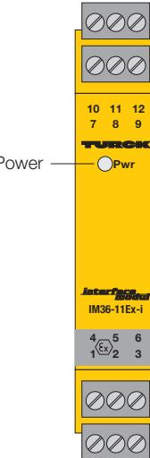
The potentiometer transducer IM36-11EX-I/24VDC isolates signals from 3-wire or 5-wire potentiometers and transfers these as standard analog signals from the Ex to the safe area. The resistance value of the potentiometer's wiper contact, ranging from 0  $\Omega$  to the nominal resistance value (final value) of the potentiometer, is detected and processed linearly (see fig.).
