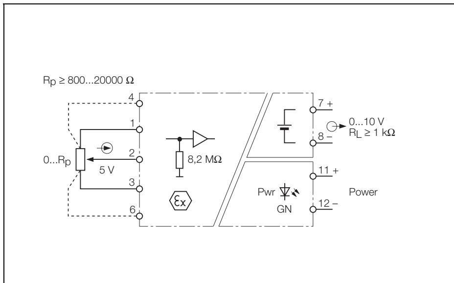
The 1-channel potentiometer transducer IM36-11EX-I/24VDC isolates signals from 3-wire or 5-wire potentiometers and transfers these as standard analog signals from the Ex to the safe area. The resistance value of the potentiometer's wiper contact, ranging from 0  $\Omega$  to the nominal resistance value (final value) of the potentiometer, is detected and processed linearly (see fig.).
